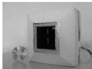
Fig 9: Measuring device with Peltier unit
