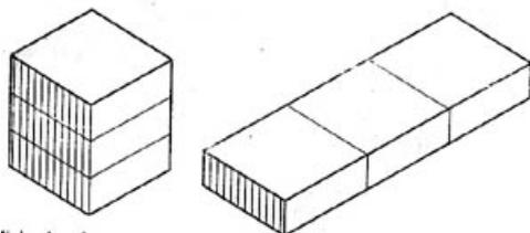
**Figure 5:** Effect of Surface area to volume ratio
