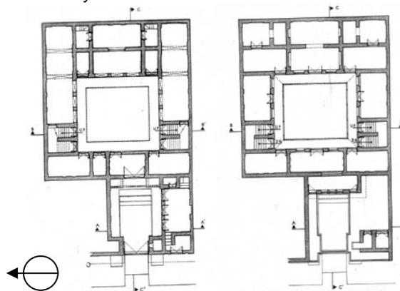
**Figure 6:** Ground Floor Plan and First Floor Plan of a Small Haveli, Dundlod, Shekhawati, Rajasthan
