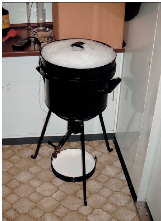
Fig. 14. The ice calorimeter in the cooling chamber. Photo: U. Drüding.
