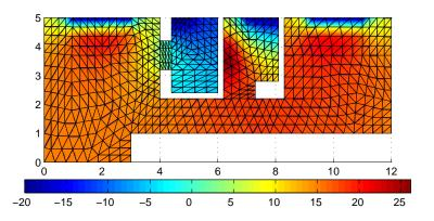
With the optimal parameter  $p^*$  from the two subdomain theory, the convergence factor ratio is in the iterative case  $32/25=1.28\approx 2^{1/3}=1.26$ , as predicted by the two subdomain theory.
