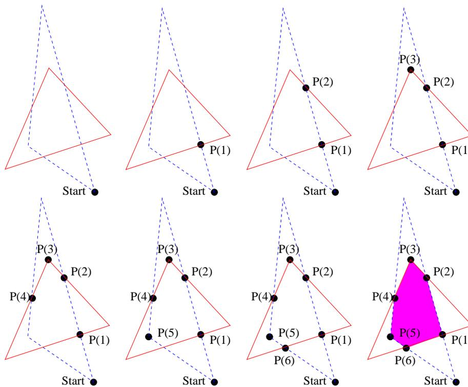
Fig. 2. Using the classical polygon clipping algorithm for computing the intersection of two triangles.
