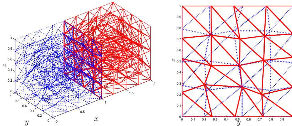
Fig. 1. Non-conforming tetrahedral discretization with two subdomains on the left, and the resulting triangular interface meshes on the right.
