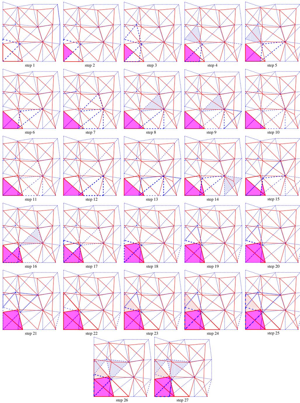
Fig. 6. First steps of an advancing front technique to compute the projection matrix for two arbitrary, non-conforming triangular meshes.
