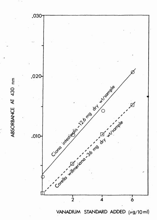
these two curves are compared simultaneously with the slope of the curve for aqueous standards (Table 6). There is no significant difference between the slopes of the three lines.
