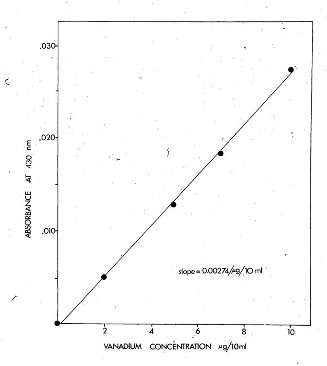
FIGURE 4. Standard additions of vanadium as vanadate to digestion solutions of <u>Ciona intestinalis</u> and <u>Corella willmeriana</u>. Preparations are reacted with phosphotungstic acid.
