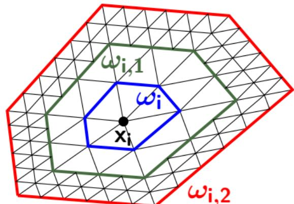
For a subdomain  $\omega_{i,2} \subset \Omega$  let  $L_{\omega_{i,2}}^{-1} : L^2(\omega_{i,2}) \rightarrow H_0^1(\omega_{i,2})$  denote the local solution operator: Given  $g \in L^2(\omega_{i,2})$ , find  $u \in H_0^1(\omega_{i,2})$  such that
