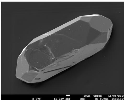
Scanning electron microscope image of a zircon. The length of the crystal is about the same as the diameter of a human hair (100 micrometers). Copyright: U. Schaltegger, J.F. Wotzlaw, R. Martini, A. Martignier
