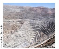
The Chuquicamata open pit mine (Chile) exploits one of the largest porphyry copper deposits in the world: it is 4.3 km long, 3 km wide and up to 0.9 km depth.
