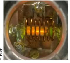
The photo shows a rare-earth crystal that serves as quantum memory. The crystal is cooled to 3 degrees above absolute zero temperature.
