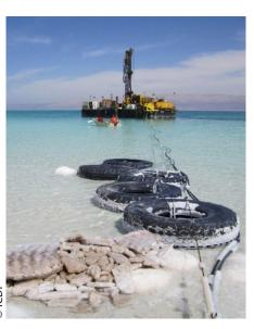
The scientific platform used to drill the sediments of the Dead Sea.
