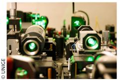
Partial view of the source producing the single photons that were stored in the quantum memory to produce entanglement between many atoms inside the memory.
