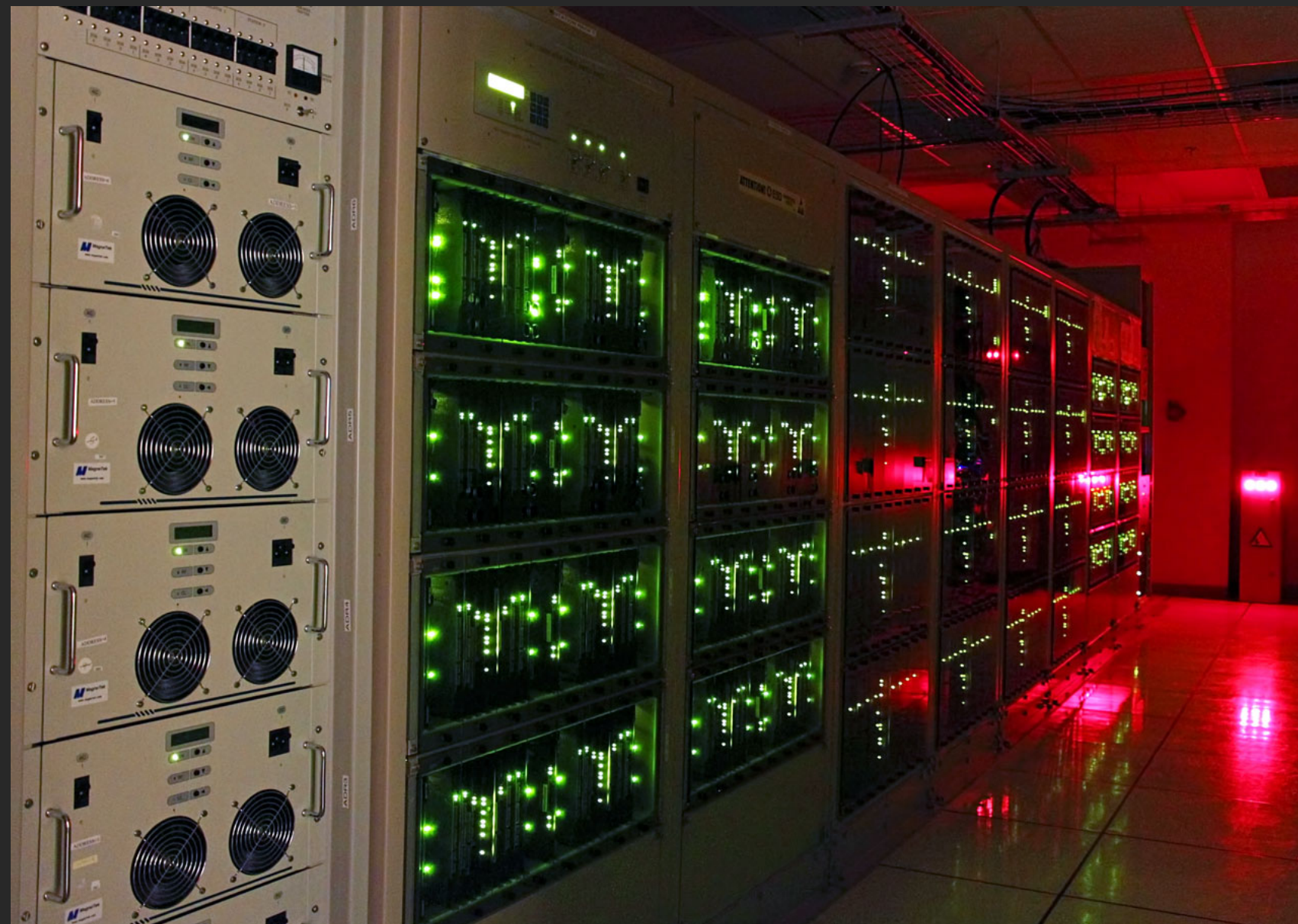
1/4 of the ALMA Correlator (3000 FPGAs in 32 racks)
