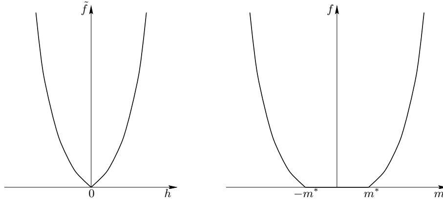
FIGURE 1. Schematic plots of the densities of the Helmholtz free energy \tilde{f} and free energy f of a ferromagnet.
