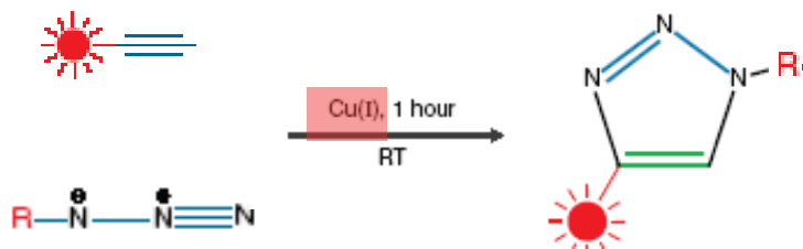
Copper catalyzed click reaction between an alkyne and an azide
