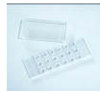
Fig 3. Sterile 18-well \mu Slide for cell cultivation for LMD.
