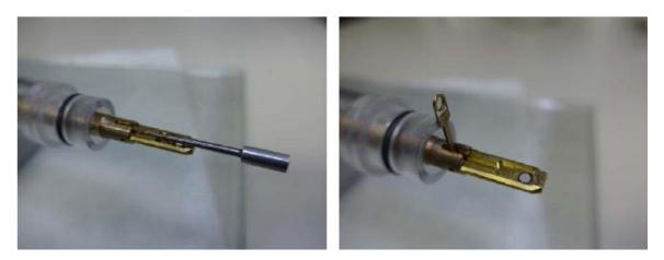
Putting the specimen holder back into the microscope (do the movements as precise as possible, never use any excessive force):
