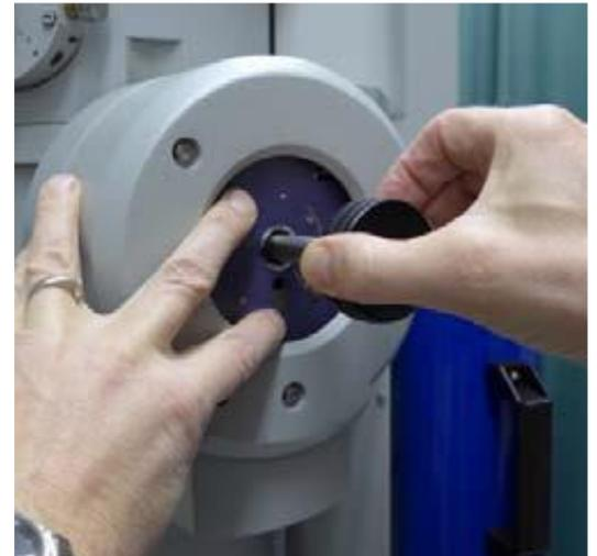
As soon as you cannot pull the holder more (but be sure to not use too much force) you turn the holder **clockwise until it stops**. The stop is after about a 120° turn and the **pin** is at a **11 O'clock** position now. (As soon as you have started the turn, the holder is stable and does not pull back so you don't need to pull anymore).
