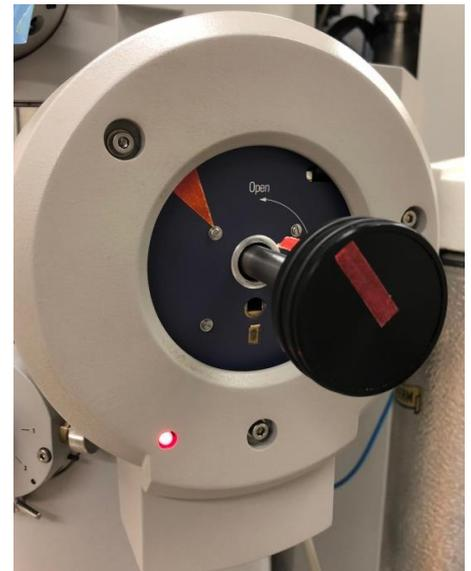
At the end of the pre-pump cycle the pump will stop and the red LD below the goniometer will get off (sometimes this LED will not go on or goes off prematurely: then you need to listen to the pump and still wait at least 90 seconds!). Now you are allowed to turn the holder slowly **anti-clockwise** until the **pin** is at the **6 O'clock position**. At this position the holder will pull in but you need to guide it slowly in until it is fully inserted.
