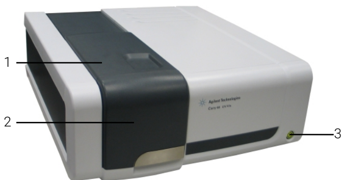
Figure 5. Cary 60 showing the sample compartment lid (1), sample compartment front door (2) and power button (3)
