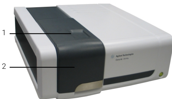
Figure 4. Cary 60 showing the sample compartment lid (1) and front door (2)
