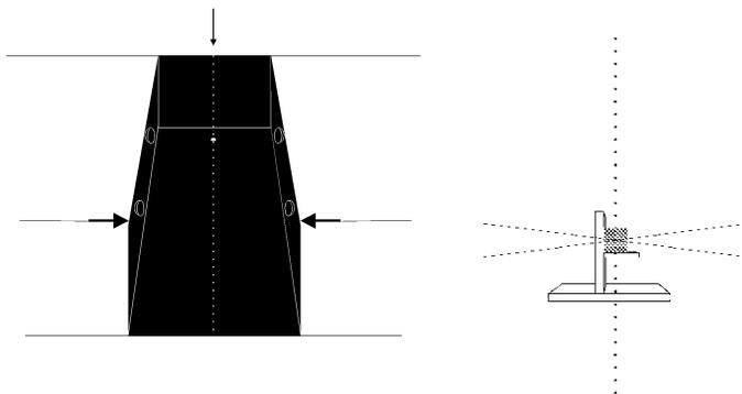
**Figure 10.** Aligning the sample in the sample compartment. Left: Sample compartment from above. The dotted line indicates the middle of the compartment. Right: Middle of the sample compartment when viewed from the side
