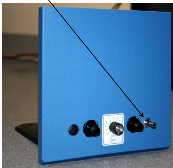
Purge port mounted on the front of the FluoroMax ® -4's sample compartment
