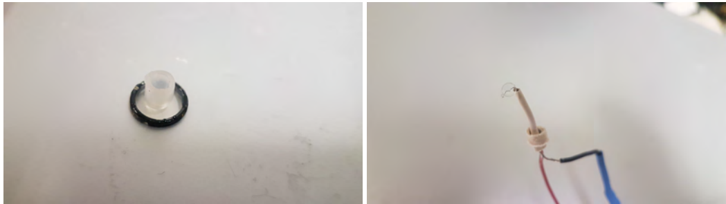
Figure 2.9: Left: Silver-embedded lens - OcuScience, of 1.5 mm radius of curvature, in Aclar, a Polychlorotrifluoroethylene homopolymer film. Right: Silver-embedded lens - OcuScience, of 1.5 mm radius of curvature, in Aclar, a Polychlorotrifluoroethylene homopolymer film.
