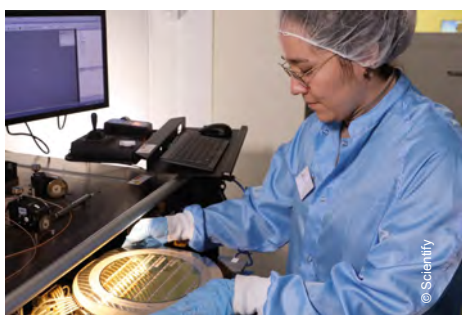
Implementation of an 8" diameter wafer with around 50 microchips, DPNC-designed, on a Cascade Microtech microprobe machine for electrical characterisation tests.
