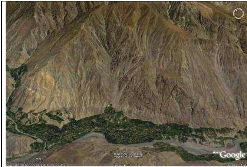
Fig: 14 Sherqila village from south-west. Debris fans develop at the bottom of a number of nallas. The slopes above the village are steep and completely dry. The eastern part of the slope immediately above the inhabited areas is much steeper than the western part. The Danjir nalla in the centre part is clearly visible. Dirani River enters from left side. Source: Google earth, accessed on 25 June 2007
