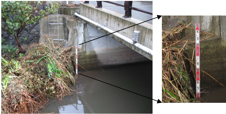
Figure 18 & 19 : The measured water level- 3.7 cm- on branch of Shirakawa River on 11 November 2006
