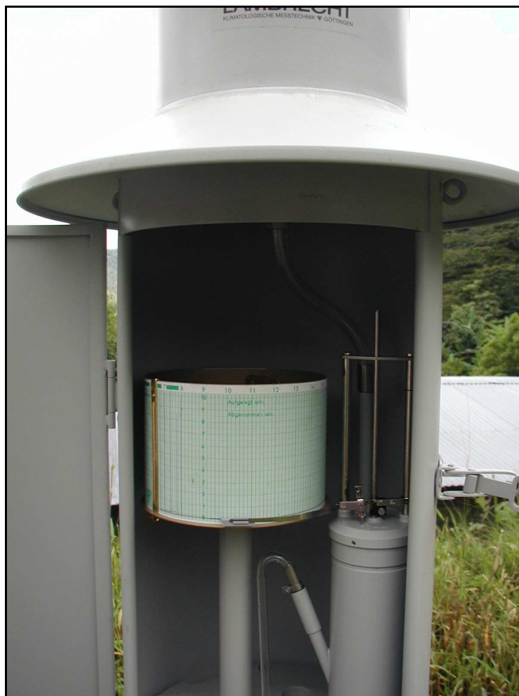
Photo 14: Detail of the pluviograph setup in El Volcan cooperative. Below the paper, is the needle which records the amount of rainfall collected in the tube as a function of the time.
