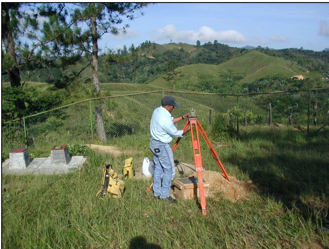
Photo 34: Installation of the tripod and the base of Leica instrument.
