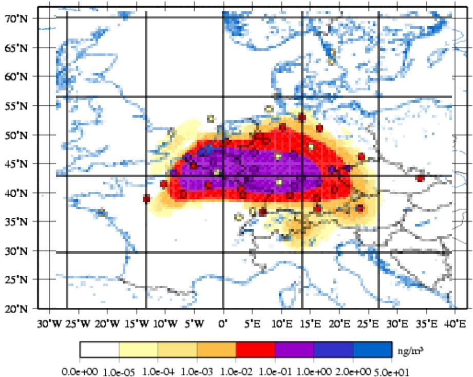
Comparison to the measurements of the ETEX1 field campaign (1994) - emission of a gas during 12h in Monterfil (Brittany, France); 168 measurement sites in Europe.
