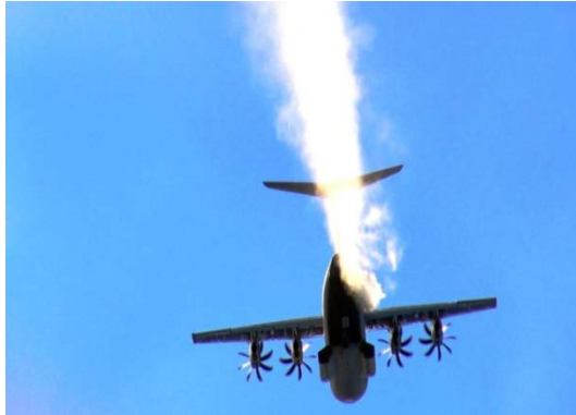
A400 M with ash plume release
