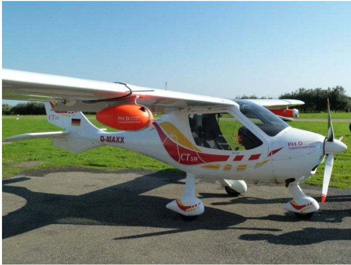
Under-wing in-situ instrumentation
