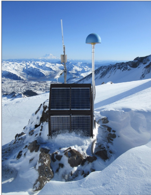
Figure B1. Photograph of monitoring station September Lobe (SEP) on the 1980–86 dome at Mount St. Helens, Washington. The site has co-located seismic, geodetic, tilt, and infrasound instruments. View is to the north; Spirit Lake is visible in the near-background and Mount Rainier is on the skyline. Photograph by Ben Pauk, U.S. Geological Survey, 2018.
