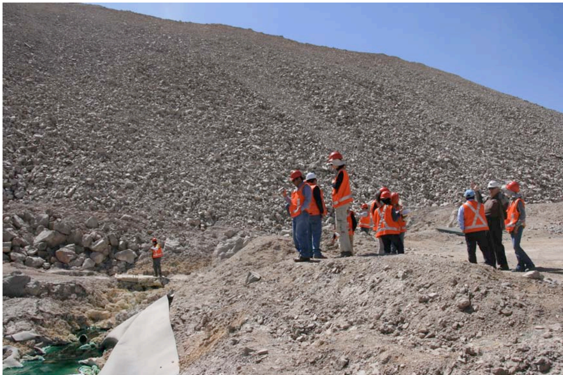
Heap (run of mine) bioleaching operation of low-grade ore at Chuquicamata (CODELCO Norte)
