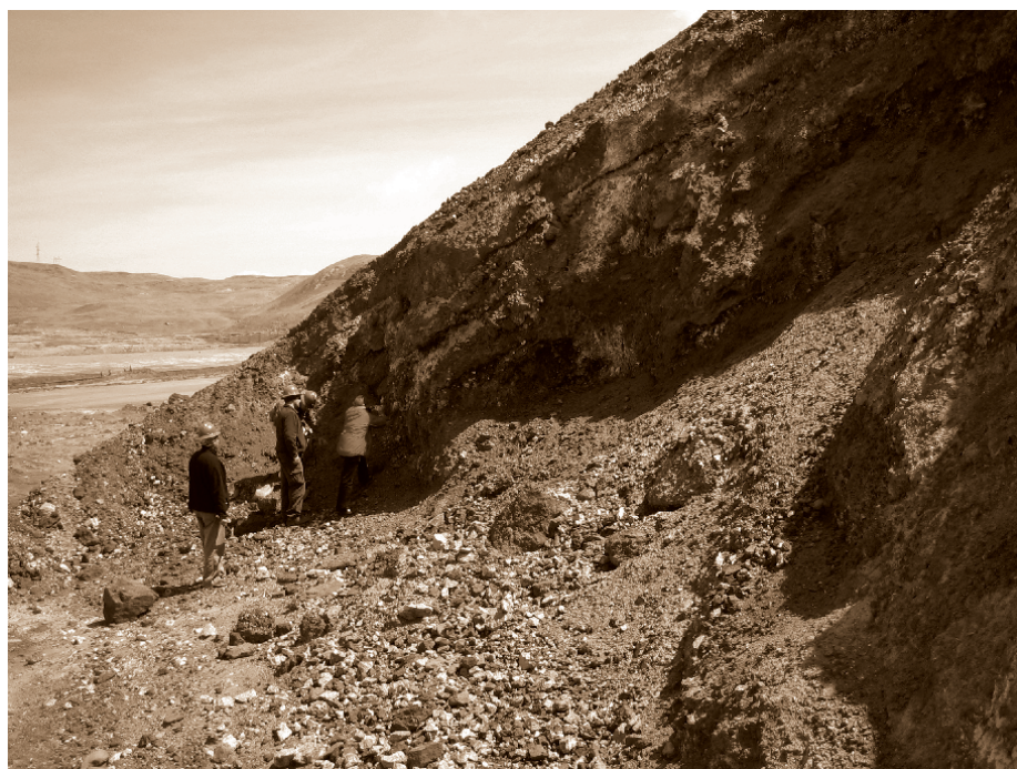
Participants studying the water flow path along the cross-bedding of the Excelsior waste-rock dump, Cerro de Pasco, Peru.
