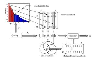
**Fig. 2**. Bit-reliability based identification decoder.
