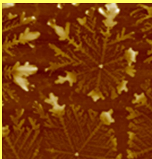
Crystallisation of chitosan-DNA hybrids on a gold surface as observed by atomic force microscopy
