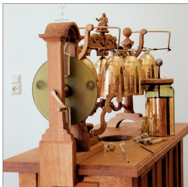
Fig. 1. Electrical machine, rebuilt as closely to Schmidt's electrical machine as possible, mainly based on Schmidt (1773).
