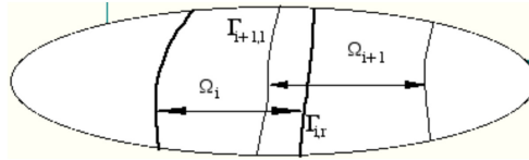
Fig. 5: Strip decomposition considered for substructured optimized Schwarz.
