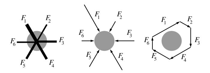
Represent the forces by linesegments perpendicular to the direction of the force with length proportional to the strength.
